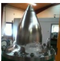
Valve without static seal
