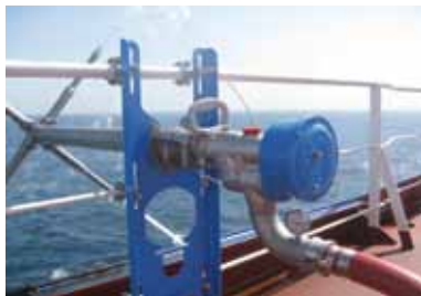
Adjustable length and angle. Easily removable. 90 degrees free bend
