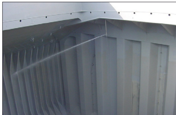
Hold cleaning process by Scanjet in a bulk carrier
