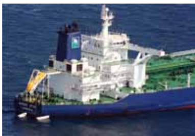
Crude oil tanker with sunken deck design
